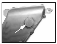
Step 7 Install the provided plug into the hole from the resonator into the fresh air duct.
