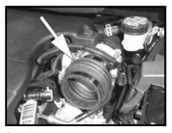
Step 10 Install the 3" flex coupler onto the throttle body and secure with the provided hose clamp. Install the second hose clamp but leave it loose for now.
