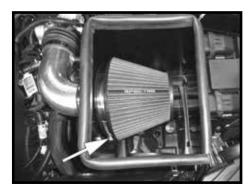
Step 14 Install the air filter onto the velocity stack and secure with the provided hose clamp.
